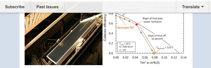
Prototype of improved flat plate collector with heat pipes during the indoor performance measurement (left) and its measured efficiency curve with characteristic power shut-off (maximum fluid temperatures < 125°C) compared to a standard flat plat collector (maximum fluid temperature of about 200°C) (right)
