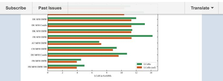
Heat costs of the solar assisted heating system (LCoHo) and their counterparts without solar assistance (LCoHo (ref)) defined within Task 54
